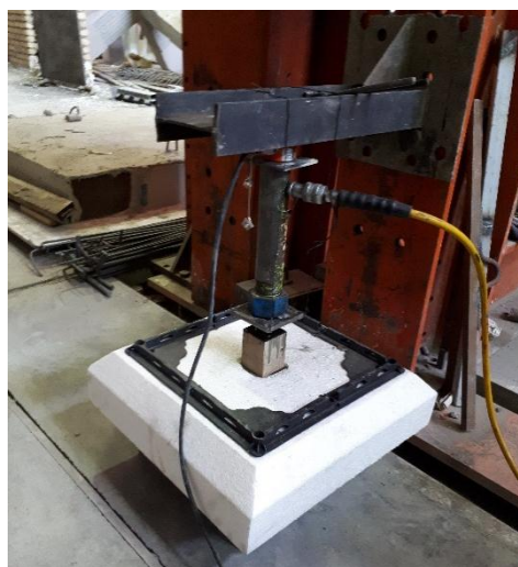
Figure 2. load applying on the center of filler
