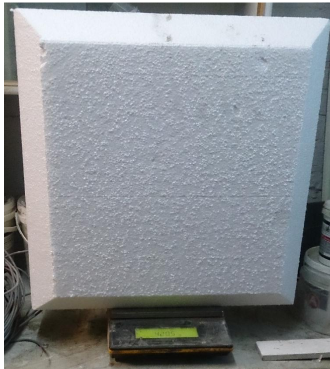
Figure 3. Weighing polystyrene block to measure density
