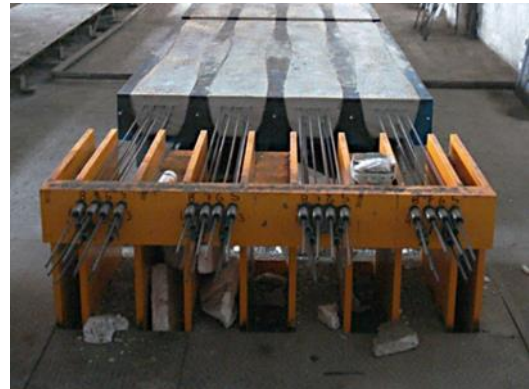
Figure 1.2. Pre-tensioning of prestressed system
